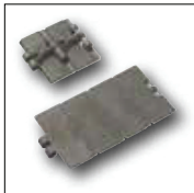
820 Single hinge Pitch 1 1/2" (38,1 mm) Thickness 4 mm (0.157") Hinge 41,6 mm (1.638")
