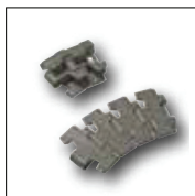
878T TAB Reinforced top Plate Reduced sideflexing radius (200 mm) Pitch 1 1/2" (38,1 mm) Thickness 4,8 mm (0.189") Hinge 42,9 mm (1.689")
