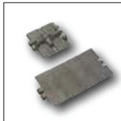
831 Single hinge Reinforced top plate Pitch 1 1/2" (38,1 mm) Thickness 4,8 mm (0.189") Hinge 41,6 mm (1.638")
