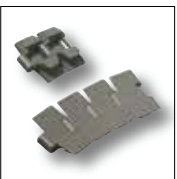
880T TAB Pitch 1 1/2" (38,1 mm) Thickness 4 mm (0.157") Hinge 42,9 mm (1.689")
